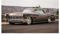
The build started with a California car and was designed and modified by the acclaimed Havasu Speed. The original frame rails were boxed and melded with a newly designed front clip from Jim Meyer Enterprises.
