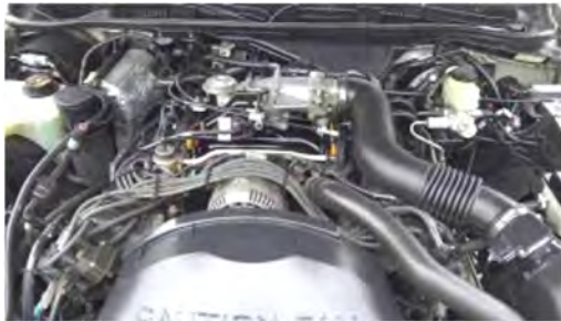
The Lincoln features a 4.6 Liter, single overhead camshaft engine, also found in Ford and Mercury automobiles.
