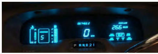
The Town Car digital instrument panel.
