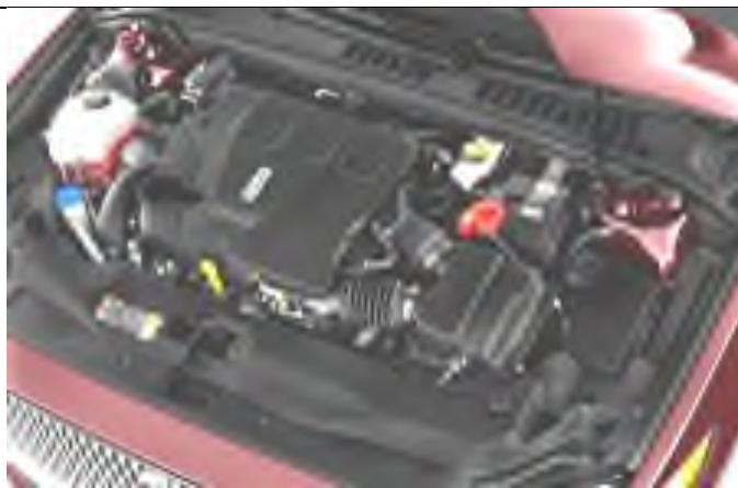
The most powerful engine in Lincoln history. The 3.0 liter 400 horsepower twin-turbocharged motor residing in the engine bay of this Lincoln Continental.
