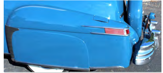
Note detail of rear quarter, gas tank lid, tail lamp, large fender skirt, front facing stone shield, "Continental spare tire." and center mounted "Cobra shaped" stop lamp.
