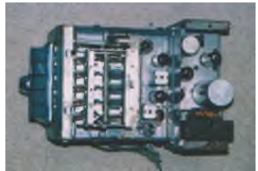
Early car radio from the 1950s featuring push button tuning and subminiature tubes.
