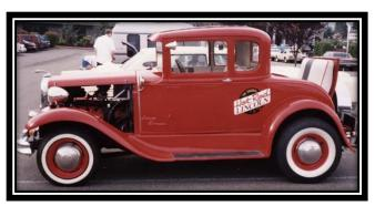
Charlie Ryan was also a car guy. In the late 1940s, he purchased a used 1941 Lincoln Zephyr four-door sedan. After a couple of years, he decided to make a hot rod out of it. He removed the Zephyr body, cut two feet off the frame to shorten the wheelbase and dropped a 1930 Ford Model A coupe body on it. At first, the car was painted black with red wheels. Charlie installed a '48 V-12 engine in it along with the 3-speed with overdrive '48 transmission.
