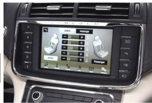
The transmission shifter is a series of vertical buttons to the far left of the touch screen system. No more gear shift selector.
