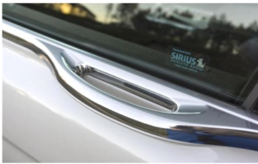
The Continental featured finely shaped door handles and were part of the E latch system.
