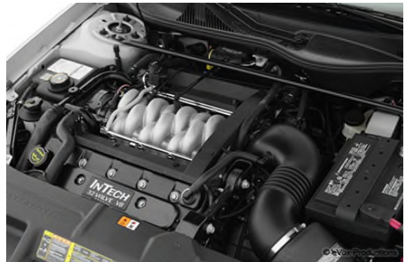
The 9th generation Continental featured the InTech 32 valve DOHC engine as their only offering.
