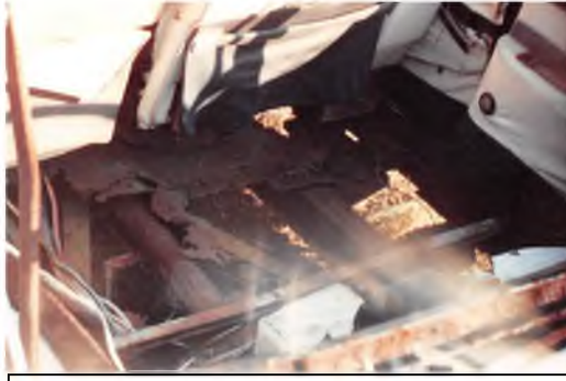
Floor panels completely rusted through.
