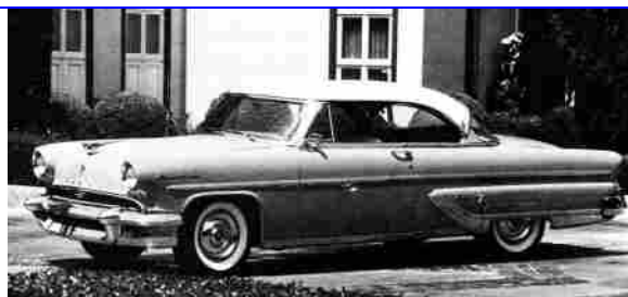
Lincoln was facelifted rather than all new for '55. In Lincoln's case it was more taillift than facelift as the rear fenders were extended for longer, lower look and new canted tail lamps were added.
