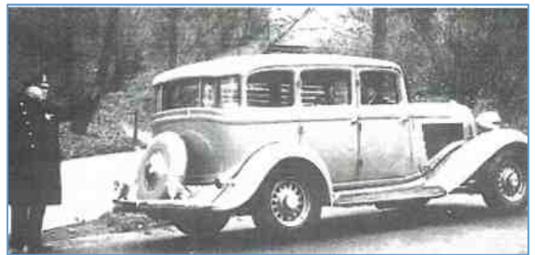
Chrysler modified a 1933 DeSoto to drive backwards to demonstrate the claim that cars of the day are more aerodynamic if driven backward.
