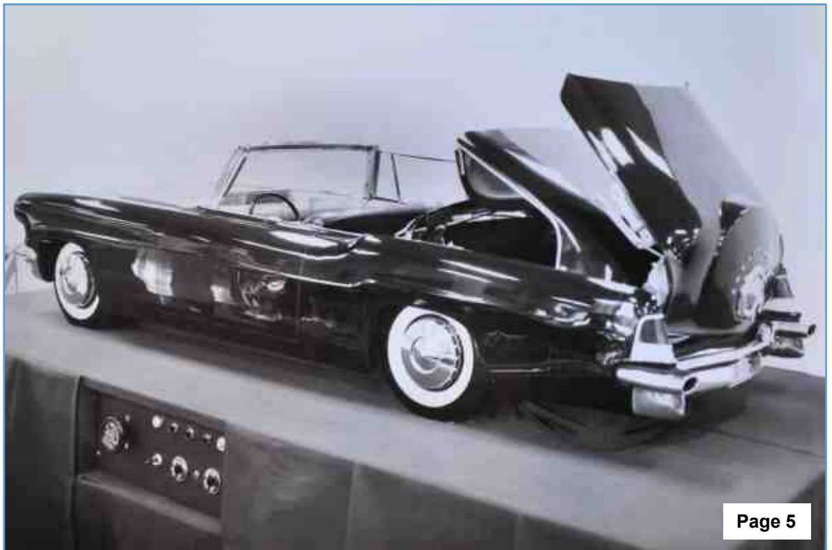
Model of retractable hardtop mechanism for Continental Mark II. Note the demonstration table and switches
