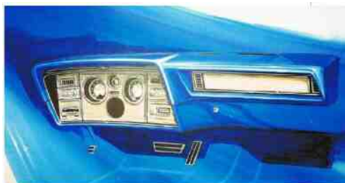
Designer Howard Payne's original sketch of the Mark IV instrument panel. It was patterned after the 1972 Ford Thunderbird; which Payne had previously designed.
