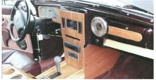
Another view of the custom interior, incorporating instruments and steering wheel from a Mark VIII. Clock is from a 1948 Continental.
