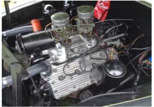
Lincoln 337 flathead engine at home under the hood of the Muntz Jet.
