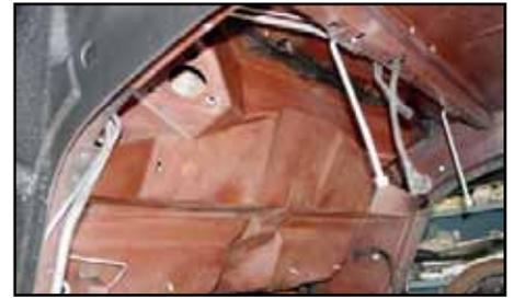
*Undercarriage in brand new condition. Hangers are for the fuel tank.*
