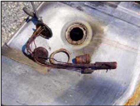
*The reason for the temporary gas can above. The gas in the tank was varnish.*
