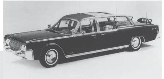
5 After JFK's assassination, the X-100 Lincoln was rebuilt as a closed limousine with a transparent top. It's shown here with the 1962 front grille and 1956 Lincoln Premiere wheel covers.
