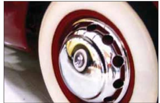
The Hub Caps which look like round discs, with holes pounded in them are exactly that. The original discs trapped so much heat that the brakes faded under severe tests.
