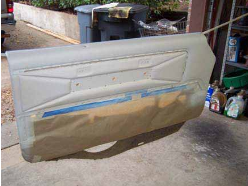
Stripped Door Panel Drying after Three Coats of SEM Color Coat Vinyl Paint. Masking Off the Lower Carpet Kick Panel Prevents Overspray. Dry Each Paint Pass Using Multiple Passes with Wife's Hair Dryer.
