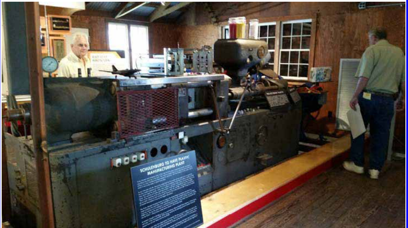
Richard Helbusch (L) and Jim Heil (R) Look Over Vintage Machine Tools. This Injection Machine was Used to Form Plastic Airplane Parts. The Original Manufacturing Shop Houses the Tools and Innovations the Stanzel Brothers Used for Model Aircraft Production.
