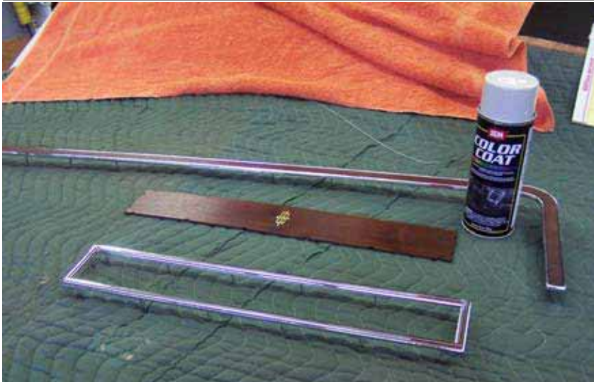
Stripped Door Panel Drying after Three Coats of SEM Color Coat Vinyl Paint. Masking Off the Lower Carpet Kick Panel Prevents Overspray. Dry Each Paint Pass Using Multiple Passes with Wife's Hair Dryer.
